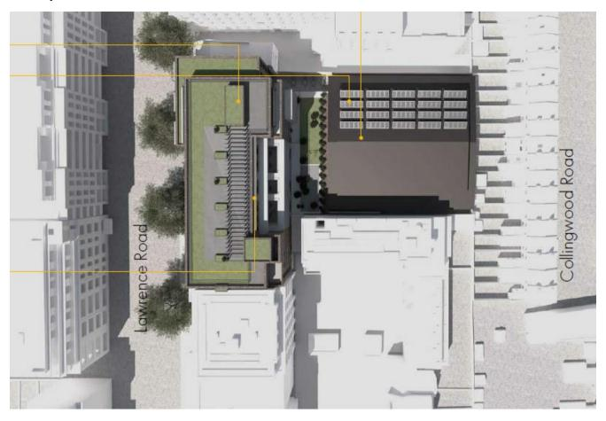
Proposal Photovoltaic panels to be relocated to existing commercial roof to allow communal space to residential roof spaces.
